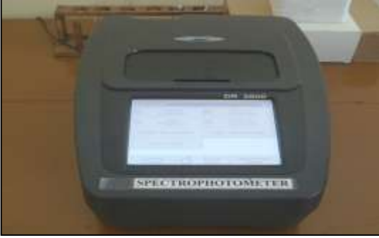
Hach Spectrophotometer: For Chemical analysis of water, sediment and soil sample
