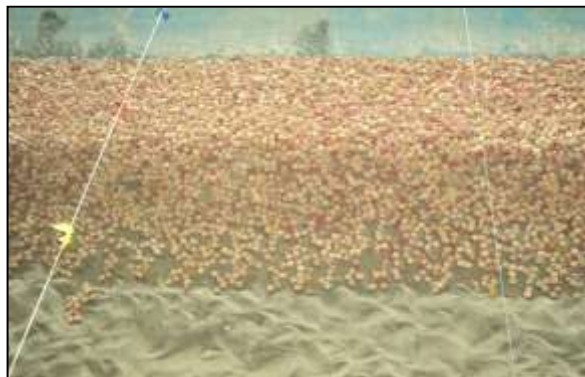
Comparison of launching pattern of geo-bags, stone-chips and CC blocks under oblique flow condition
