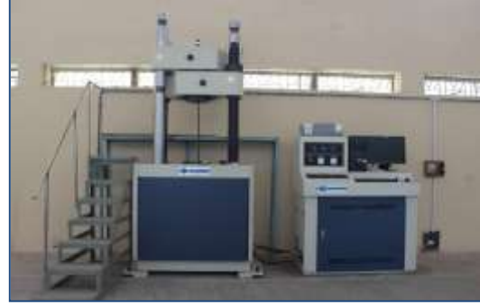
Universal testing machine used for testing of MS rod, flat bar, concrete cylinder, block etc.
